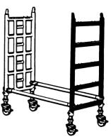
3. Fit opposite ends of short braces to other 5 rung base frame ensuring pegs on frame head fitting point towards middle of tower.
