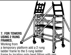
frame by locating onto head fitting with peg. engaging into hole provided. Repeat the process at the other end using a 2 rung frame. Add a diagonal brace to the top rung of the 2 rung frame on one side of the tower. Remove temporary platform and relocate onto 5th rung of base frame. Fit short braces to form guardrails as before.
