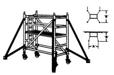
5. Fit appropriate stabilisers (see schedule on back page) to each corner of the tower to increase the effective base dimensions A & B. They must be fitted so that when viewed from above the largest square is formed. Ensure the wing nuts are tight so that it is not possible to move stabilisers without slackening the wing nuts.
