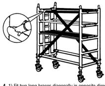
4. 1) Fit two long braces diagonally in opposite directions as close to the frame vertical tube as possible. 2) Fit a temporary platform on the third rung down from the top of the frame and, working through the trap fit short braces as temporary handrails onto frame uprights above top rungs of frames. At this stage level the tower by adjusting collar on castors (see notes)
