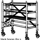
**4.** 1) Fit two blue or black braces (for a 1.8m tower fit blue and a 2.7m tower fit black) diagonally in opposite directions as close to the frame vertical tube as possible. 2) Fit a temporary platform on the third rung down from the top of the frame and, working through the trap fit two short braces as temporary handrails onto frame uprights above top rungs of frames. At this stage level the tower by adjusting collar on castors (see notes). Continue as (5-12) on opposite page.
