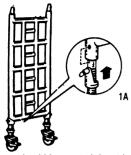
1. These towers should be erected by at least 2 competent persons. Contact your supplier for details of appropriate training. Check you have the correct equipment and it is in working order. Apply brakes and fit adjustable castors into both 5 rung frames ensuring that spring loaded pin is engaged in hole provided (see detail 1A).
