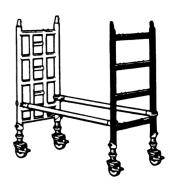
**3.** Fit opposite ends of short braces to other 4 rung frame ensuring pegs on frame head fitting point towards middle of tower.
