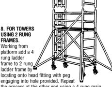
the process at the other end using a 4 rung main frame. Working through the trap fit 4 short braces as guardrails fit two braces diagonally in opposite directions as close to the frame vertical tubes as possible
