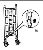
1. These towers should be erected by at least 2 competent persons. Apply brakes and fit adjustable castors into one 4 rung ladder frames and one 4 rung main frame, ensuring that spring loaded pin is engaged in hole provided (see detail 1A).
