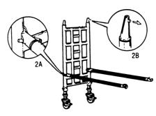
2. Make sure pegs on frame head fitting always point towards middle of tower (see detail 2B). Fit two short horizontal braces to vertical tubes of one of the frames ensuring spring loaded pin faces outwards (see detail 2A).
