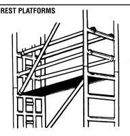
Rest platforms must be fitted every 2m and consist of a trap platform and guardrails at 1m as shown. Remember to always close trapdoor immediately after climbing through.
