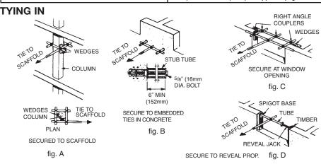
NOTE: Arrangement shown in fig. D is considered to be a friction device and should not exceed  $\frac{1}{2}$  the total number of scaffold ties in any area.
