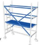
4.) Fit two blue (1.8m tower) or black braces (2.7m tower) diagonally in opposite directions as close to the frame vertical tube as possible. 2
