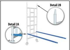
2. Make sure pegs on frame head fitting always point towards middle of tower (see detail 2B). Fit two short horizontal braces to vertical tubes of one of the frames ensuring spring loaded pin faces outwards (see detail 2A).
