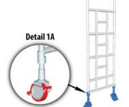
1. These towers should be erected by at least 2 competent persons. Apply brakes and fit adjustable castors into one 4 rung ladder frames and one 4 rung main frame, ensuring that spring loaded pin is engaged in hole provided (see detail 1A).
