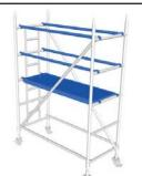
3. 1) Fit two long braces diagonally in opposite directions as close to the frame vertical tube as possible. 2) Fit a temporary platform on the 3rd rung down from the top &, working through the trap, fit short braces as temporary handrails onto frame uprights above top rungs of frames. At this stage level the tower by adjusting collar on castors (see notes).
