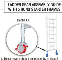
1. These towers should be erected by at least 2 competent persons. Contact your supplier for details of appropriate training. Check you have the correct equipment and it is in working order. Apply brakes and fit adjustable castors into both 5 rung frames ensuring that spring loaded pin is engaged in hole provided (see detail 1A).
