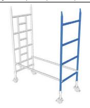
3. Fit opposite ends of short braces to other 4 rung frame ensuring pegs on frame head fitting point towards middle of tower.
