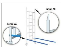
2. Make sure pegs on frame head fitting always point towards middle of tower (see detail 2B). Fit two short horizontal braces to vertical tubes of one of the frames ensuring spring loaded pin faces outwards (see detail 2A). Repeat with a 5 rung frame at the opposite end.
